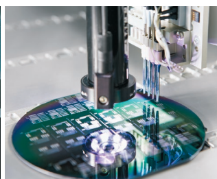
Microscope for optical target recognition and adjustment
