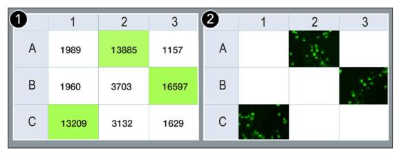
(1) Plate reader quickly identifies GFP positive wells. (2) Only GFP positive wells are imaged, saving both time and computer memory.
